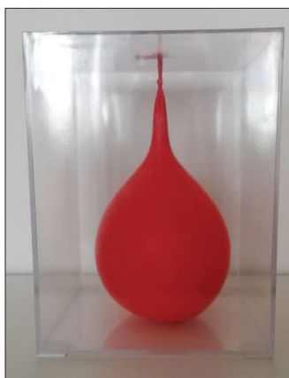
Fig. 1. The extended neck of the water-filled balloon indicates that the balloon has weight.
