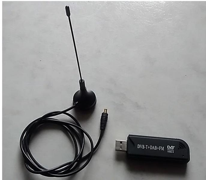
**Figura 9:** Dongle RTL - SDR
