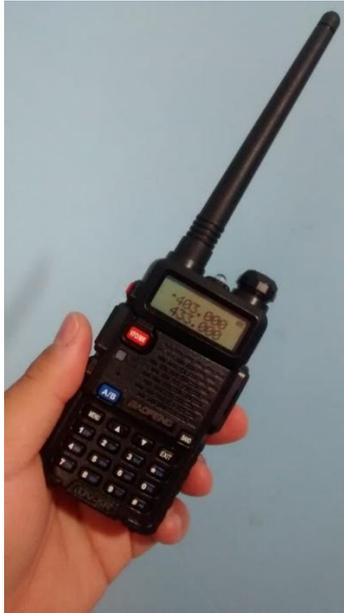
**Figura 8:** Radio transceptor da Baofeng modelo UV-5R
