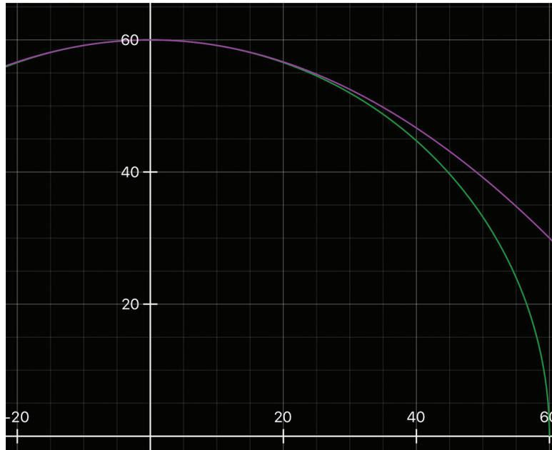
**Figure A1.** The green curve represents 1/4 of the circular orbit of the Moon:  $y = \sqrt{60^2 - x^2}$  with  $x \in [0, 60]$ . The red curve represents the parabolic approximation  $y \approx 60 - x^2/120$ . For both axes the measure unit is the radius of the Earth  $R$ .
