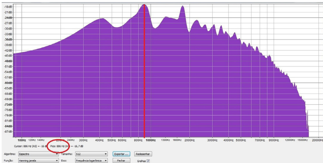
Figure 3. Spectral analysis of sound wave in region B (the source moving toward the receiver). The red line on the graph marks the average value.
