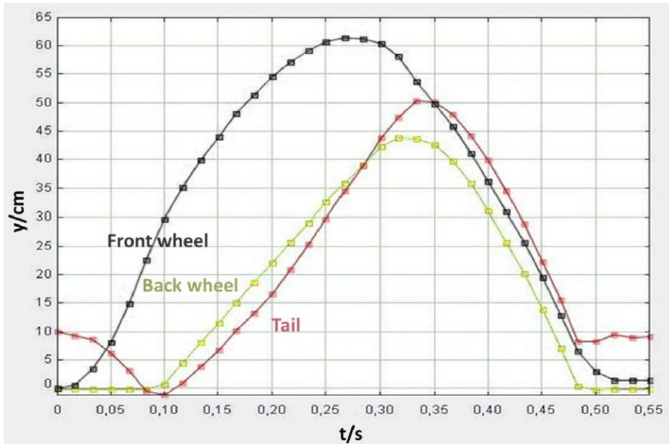
Figure 4. Superposition of plots of y-position versus time for three points of the skateboard: the tail, the rear wheel and the front wheel.
