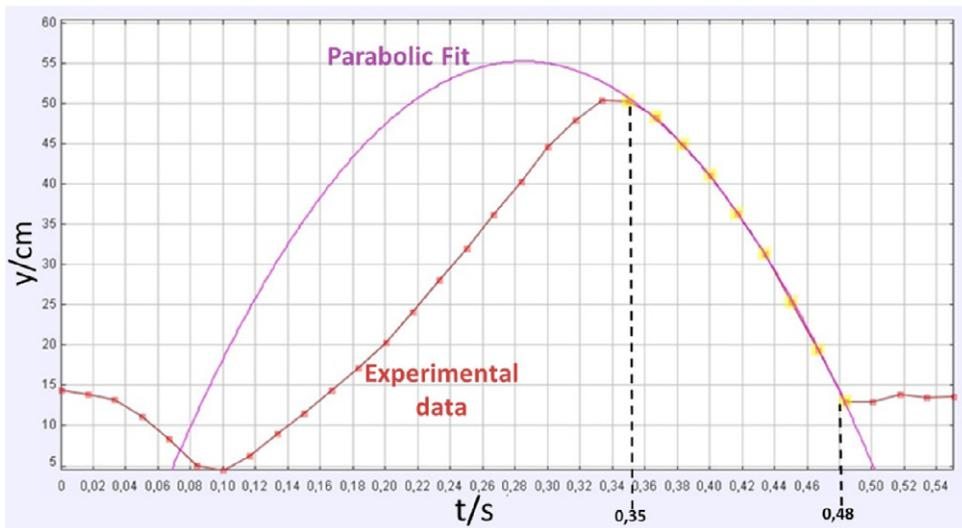
Figure 5. Experimental data for position versus time of the tail of the skateboard. Between  $t = 0.35$  s and  $t = 0.48$  s, a parabolic curve of equation  $y(t) = -12.08t^2 + 6.89t - 0.42$  (m) fits data quite well, indicating a movement with a constant acceleration of about  $24.2 \text{ m s}^{-2}$ , considerably greater than the gravitational acceleration.
