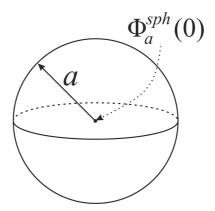
Figure 2. Sphere of radius a charged with a uniform volume charge density  $\rho$ . The electrostatic potential at the center of the sphere is denoted by  $\Phi_a^{sph}(\mathbf{0})$ .
