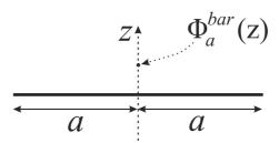
Figure 4. Bar of length 2a uniformly charged with linear charge density  $\lambda$ . The electrostatic potential at a generic point of the positive  $\mathcal{OZ}$  semi-axis is denoted by  $\Phi_a^{bar}(z)$ .
