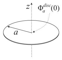
Figure 3. Disc of radius a charged with a uniform surface charge density  $\sigma$ . The electrostatic potential at the center of the disc is denoted by  $\Phi_a^{disc}(\mathbf{0})$ .
