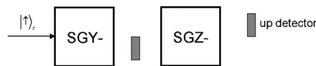
Fig. 10. Sketch of the Stern–Gerlach apparatus, initial spin state, and detectors for Question 4.
