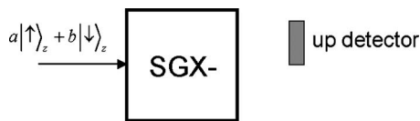
Fig. 12. Sketch of the Stern–Gerlach apparatus, initial spin state, and detector for Question 7.
